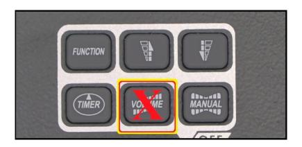
**Step 7:** When operations are complete, stop the flow of fog by pressing the "MANUAL" button once. Turn the machine off using the red on/off switch. Pull back on the yellow tab, turn counter-clockwise, and remove the power cord. Fold and stow the power cord in the handle of the reservoir tank.
